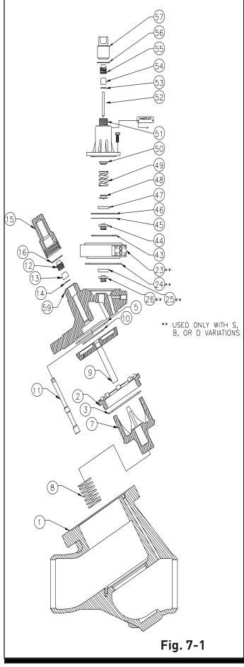
Clean the sealing surfaces where the Adapter-to-Body Gasket 5 is to beinstalled and insert a new Gasket in position, making sure to line up the hole in the Gasket with the passage "N" hole (see Fig. 1) in the Valve Body 1. The gasket should have a very light film of refrigerant oil applied to both surfaces before inserting in place.
