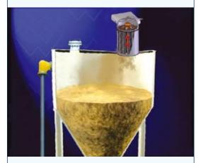
Dust drops down into the silo due to vibrating filter elements
